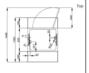
Electric Supply voltage: 322021 (F02H2AW04S) 220-240 V/1N ph/50/60 Hz Electrical power max.: 2.32 kW Water: Drain line size: 3/4" **Key Information:** N° of doors: External dimensions, Width: 800 mm External dimensions, Depth: 1180 mm External dimensions, Height: 1304 mm Net weight: 97.5 kg Shipping height: 1334 mm Shipping width: 840 mm 899 mm Shipping depth: Shipping volume: 1.01 m<sup>3</sup> Set temperature: +25 / +35 °C
